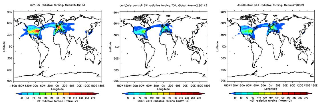
Figure 2 – Long Wave, Short Wave and NET (LW +SW) radiative forcing maps of contrail forcing (the colourbar in the SW map uses the absolute value of the forcing).
