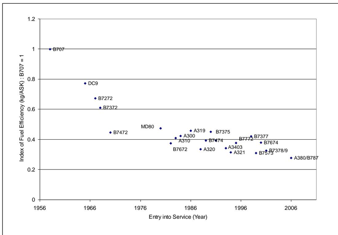
Figure 6. Fuel efficiency trend by aircraft Entry into Service date (from 1959) weighted for actual distance travelled (from FAST 2000 data)
