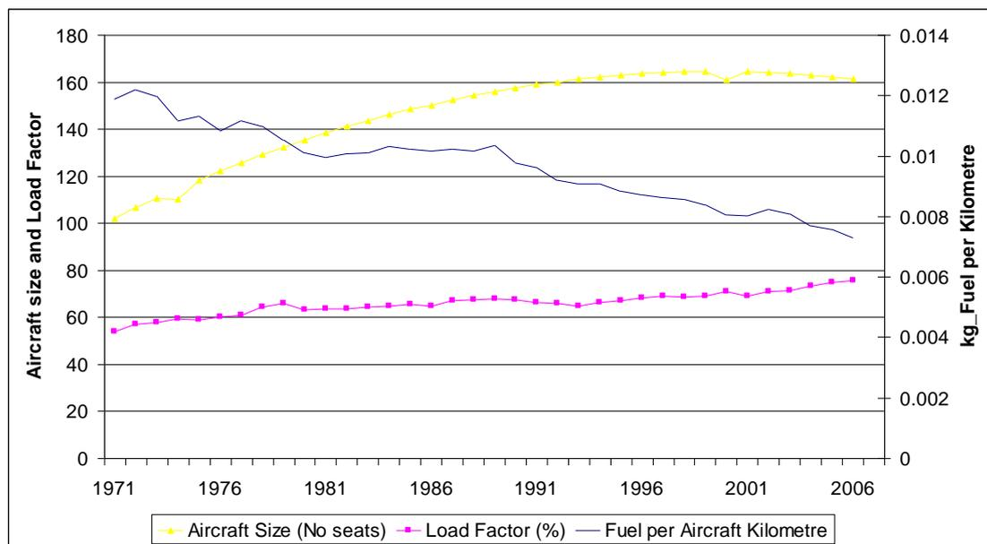
Figure 4. Estimation of Aircraft Size (number of seats), Load Factor (%) and Mass of Fuel (kg per aircraft kilometre) from Air Traffic Statistics
