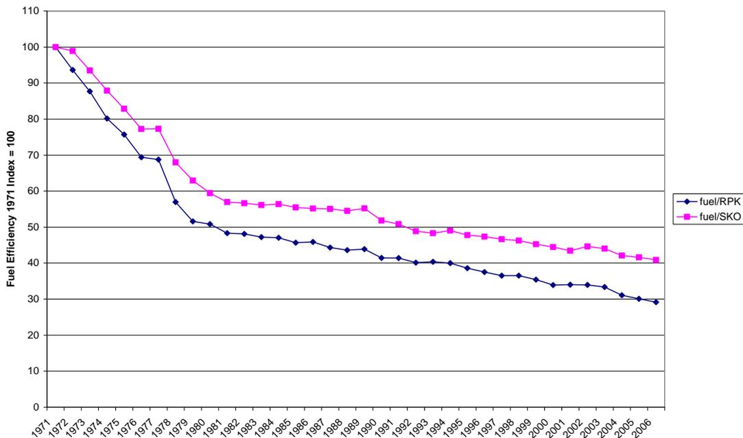
Figure 2. Trends in Global Aviation Fleet Fuel Efficiency (mass of fuel per ASK or SKO and RPK) from 1971 to 2006
