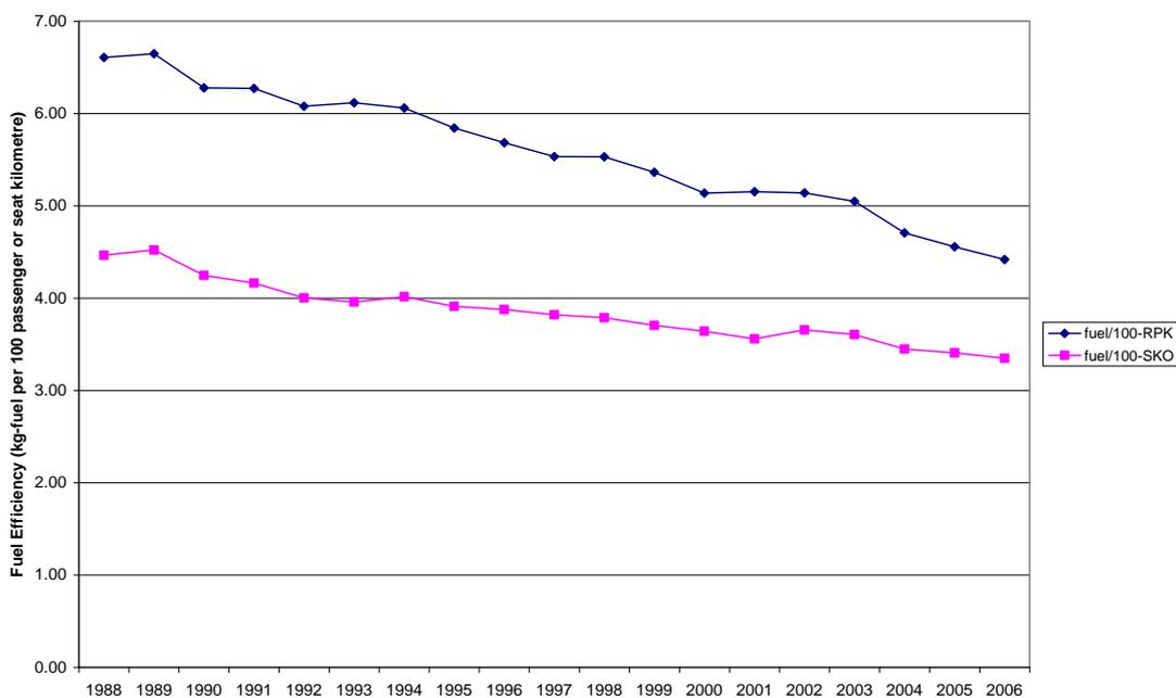
Figure 3. Calculated Global Fleet Fuel Efficiency Values from Global Fuel and Air Traffic Statistics (1986- 2006).
