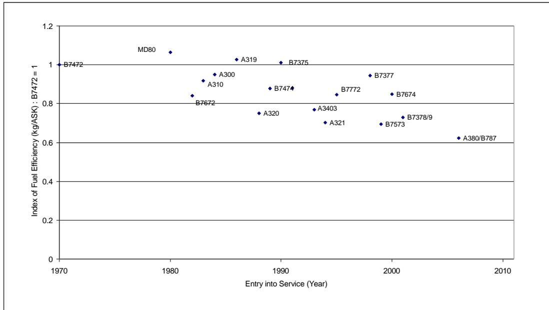
Figure 7. Fuel efficiency trend by aircraft Entry into Service date (from 1970) weighted for actual distance travelled (from FAST 2000 data)
