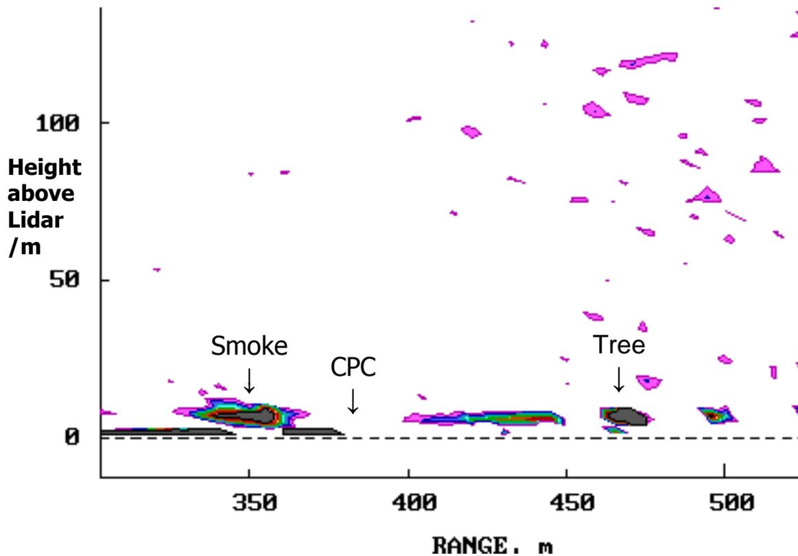
**Figure A7** Particle number concentrations for the final sortie from the condensation particle counter (CPC) beside the SPARCLE. These seem to arise almost exclusively from the engine smoke. The first spike is from the aircraft taxiing out; the second from the take-off run; and the third from landing. The Lidar detected a compact puff of tyre smoke which would have passed through the range of the CPC detector at 14:15:32.
