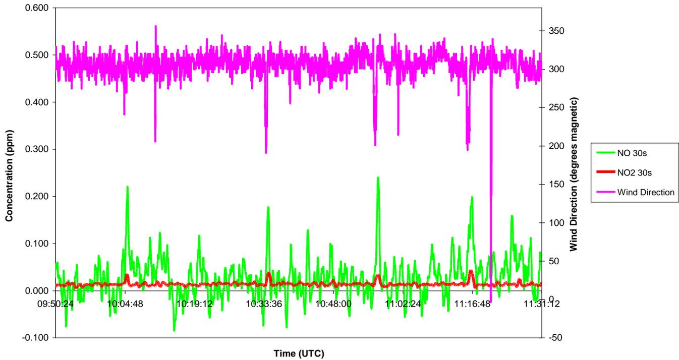
**Figure A3** Osiris wind direction and NO<sub>x</sub> & CO from Type A monitor in centre of far array, Sortie 7. The third spike of wind direction is from a light aircraft coming in to land.
