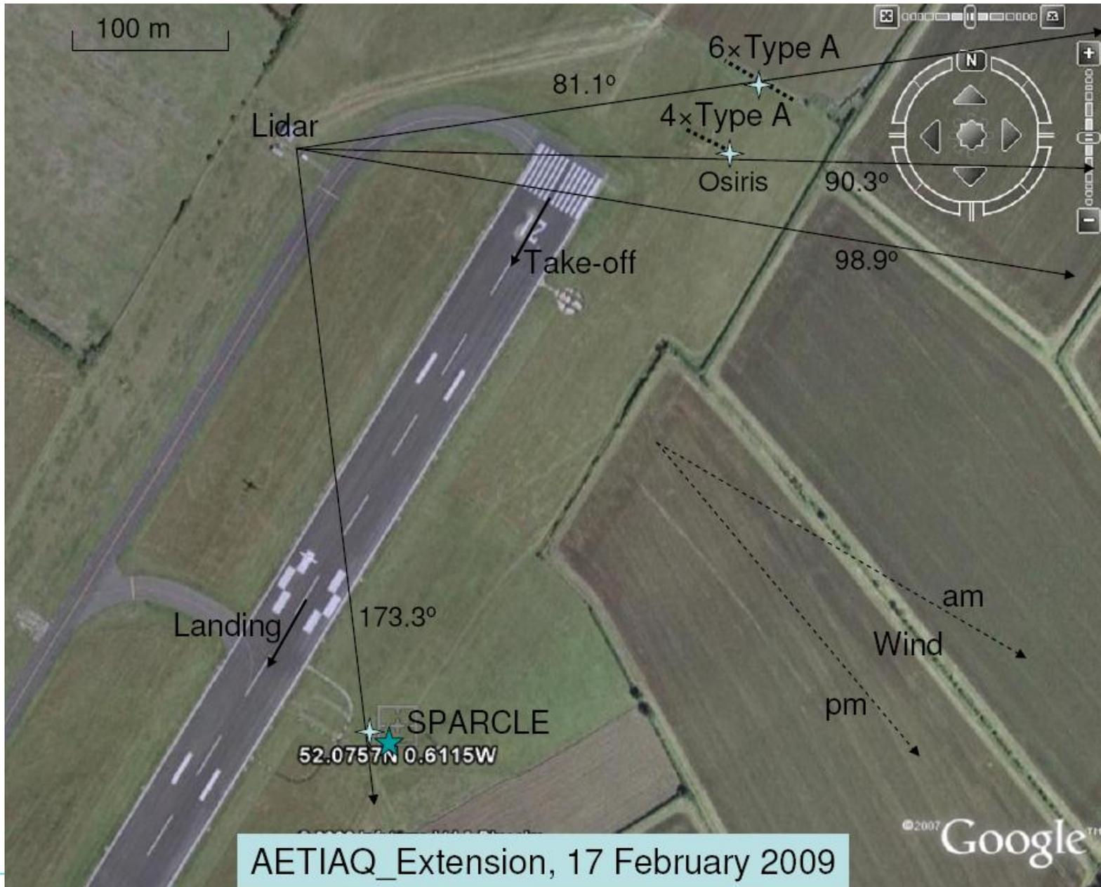
Figure A1 Layout of instruments for AETIAQ Extension study.
