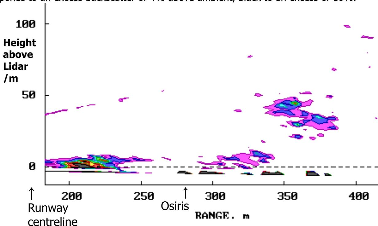
**Figure A6** Lidar cross-section of tyre smoke from touch-down at the end of the last sortie. Time 14:15:29. Azimuth 173.3°. The aircraft touched down at 14:15:07. The smoke at this point would have travelled about 60 m from the point of release. The lowest contour corresponds to an excess backscatter of 5% above ambient, black to an excess of 35%.
