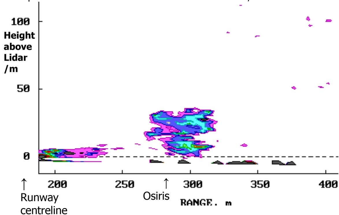
**Figure A5** Lidar cross-section of take-off exhaust plume. Time 14:10:53. Azimuth 90.3°. The aircraft powered up at about 14:10:27 and started moving at 14:10:43. The lowest contour corresponds to an excess backscatter of 4% above ambient, black to an excess of 16%.
